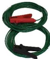
Potential cables: Channel 2
